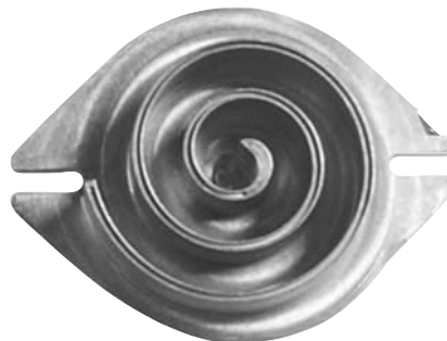
One of two matched scroll plates — the distinguishing feature of the scroll compressor.
